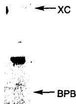
Fig. 7 Electrophoresis of the octamer (Fig. 6-II) on a 20% polyacrylamide gel containing 7 M urea, visualized by UV-shadowing.
